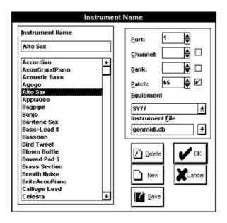
Multiple instrument sets can be defined and saved in seperate instrument files. Cadenza for Windows comes with two instrument files one is call instrumt.db. It is actually does not contain any instruments. The other is called genmidi.db. It contains the 128 General MIDI patches.
